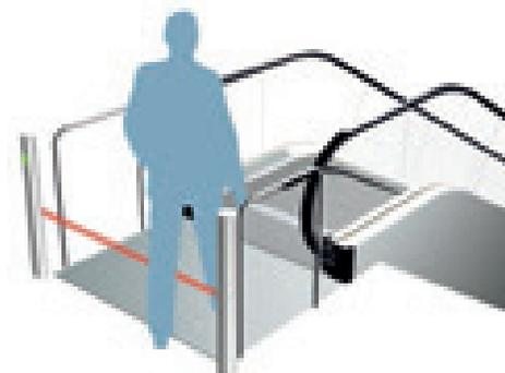
*Figure 5.8 Passenger detection by radar or a photocell*
