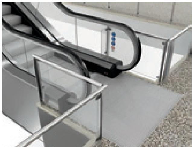
Figure 5.11 Standard arrangement without extended balustrade requires 90° static railings to be installed for safety reasons
