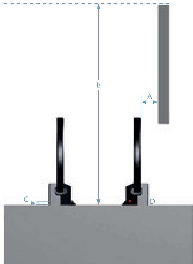
Figure 6.3 Minimum free area around escalators and autowalks
