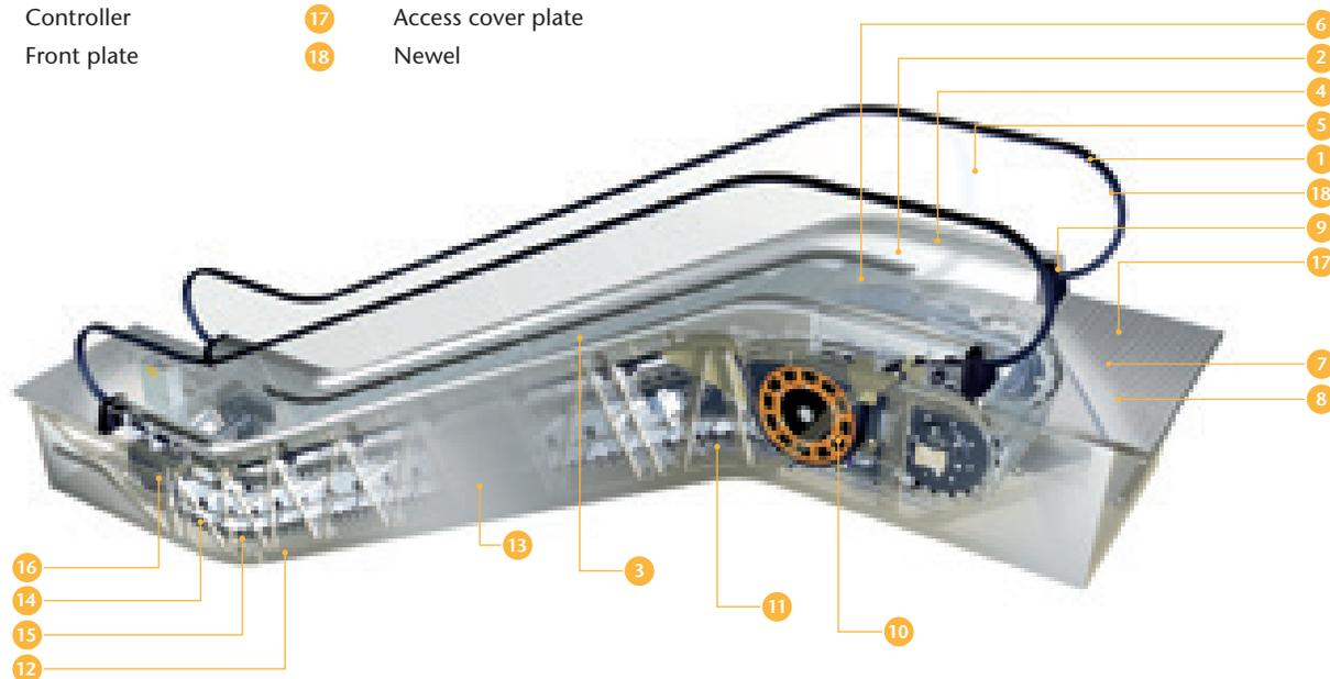
Figure 3.1 Escalator components
