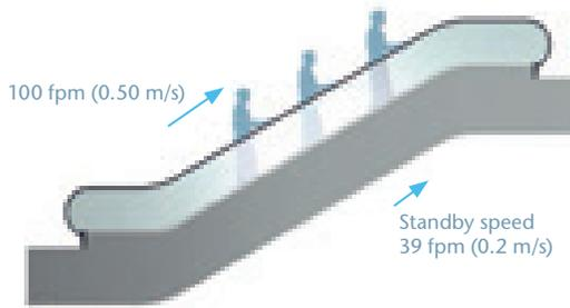
Figure 5.6 The nominal speed for escalators and autowalks
