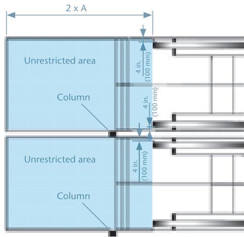
Figure 6.2 Passenger circulation area for parallel escalators
