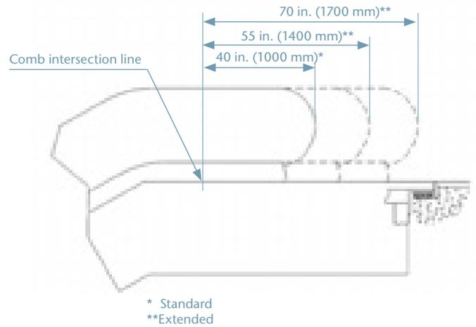
Figure 5.13 Different extended balustrade lengths
