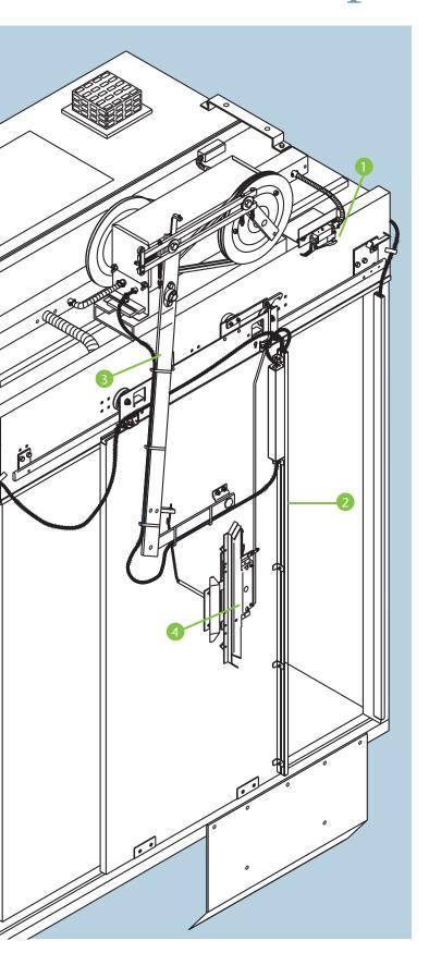
The MAC Closed-Loop Door Operator is a permanent-magnet solid-state and closed-loop operator which provides consistent high-performance door operation for all types of applications.
